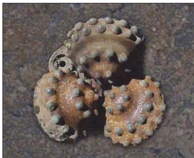
The wear on the cutting structure (bit gauge loss) of the 8½-in. CH55MRS bit No. 196982 was about 1 mm (Fig. 10).
