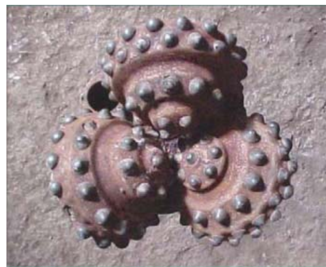
This 8½-in. CH55MRS bit, No. 191084, made 521 m of hole in 52.5 hr in Well No. 30005 in the Vostochno-Suleyevskaya area (Fig. 4).
