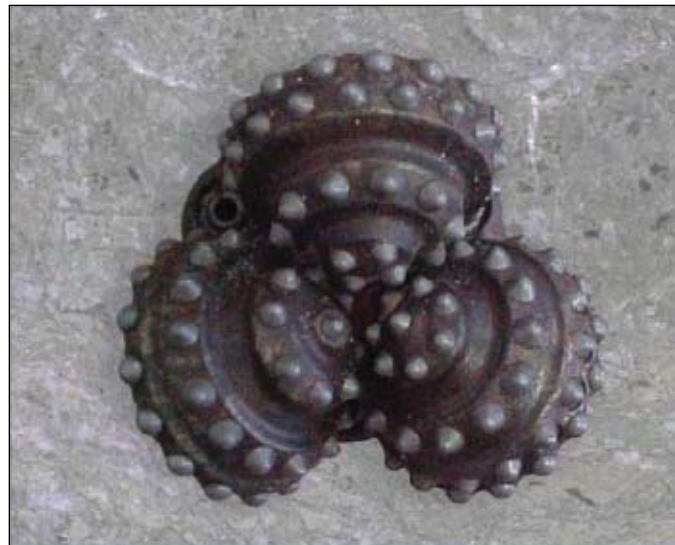
This 8½-in. CH55MRS bit, No. 191103, made 436 m of hole in 42 hr in Well No. 12024 in the Sarmanovskaya area (Fig. 6).
