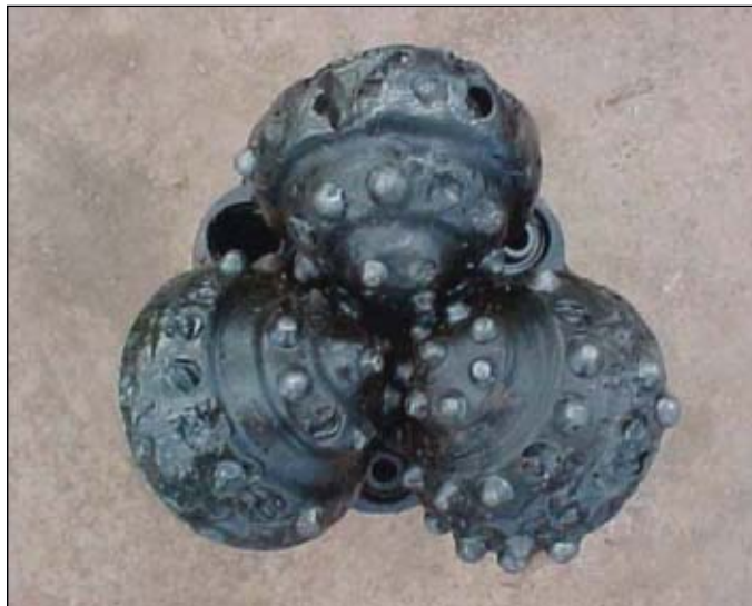
The same bit as shown in Fig. 4, after its second run in Well No. 24594 in the Aznakayevskaya area, after drilling an additional 555 m in 55 hr. In total, this bit penetrated 1,076 m in 107.5 hr at an average ROP of 10 m/hr (Fig. 5).
