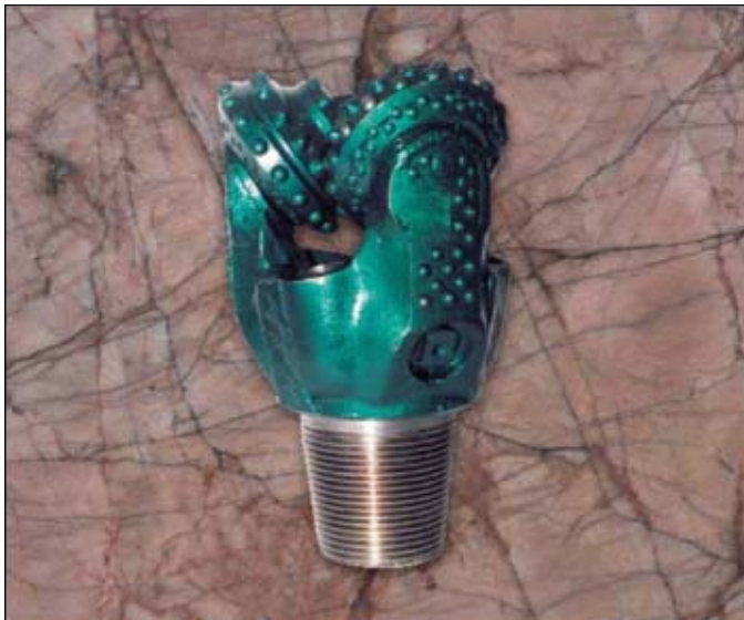
This Challenger-type, 8½-in. CH55MRS (IADC code 637Y) jet roller cone bit has sealed oil-filled bearings and is used for drilling hard abrasive formations (Fig. 1).
