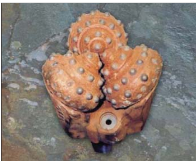
A bit from another manufacturer was dull after drilling 539 m in 48.7 hr at ROP 11.1 m/hr in the Berezovskoye field, Tatarstan (Fig. 3).
