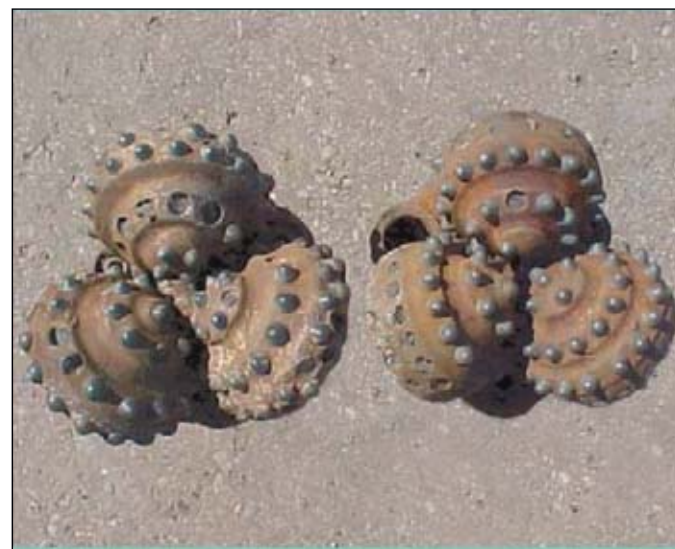
The 8½-in. CH55MRS bit No. 191103 is shown at left after making 854 m of hole in 117 hr. A corresponding bit, produced by another manufacturer, is shown with diamond inserts at the outer end of the cones (right) after drilling 868 m in 82.2 hr in the Aznakayevskoye drilling department area at the average ROP of 10.5 m/hr (Fig. 8).
