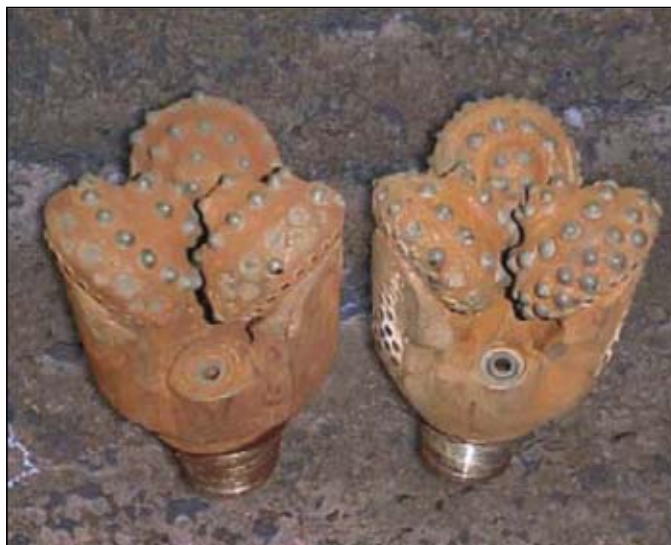
The 8½-in. CH55MRS bit No. 191083 is shown at right after making 690 m of hole in 59.5 hr at ROP 11.6 m/hr using the high-speed (240 rpm) positive-displacement downhole motor in the Almet'yevskaya drilling department area. A corresponding bit, produced by another manufacturer (left), drilled 592 m in 52 hr in the same area at ROP 11.4 m/hr using the low-speed (100 rpm) downhole motor (Fig. 9).
