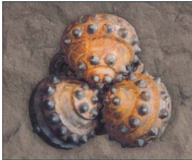
The cone heel rows exhibited premature wear while the bit bearing remained in operable condition (Fig. 2).
