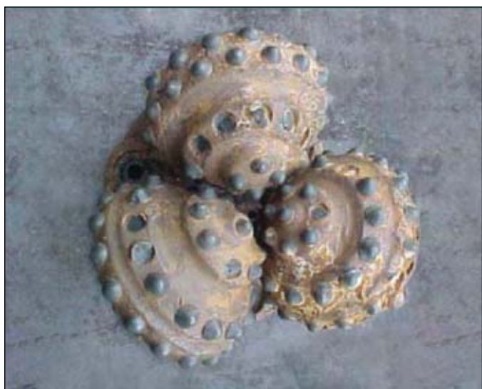
The same bit as shown in Fig. 6, after its second run in exploratory Well No. 40100 in the Tumutukskaya area, after making an extra 418 m of hole in 75 hr. In total, the bit penetrated 854 m of hole in 117 hr in two runs at an average ROP of 7.3 m/hr (Fig. 7).
